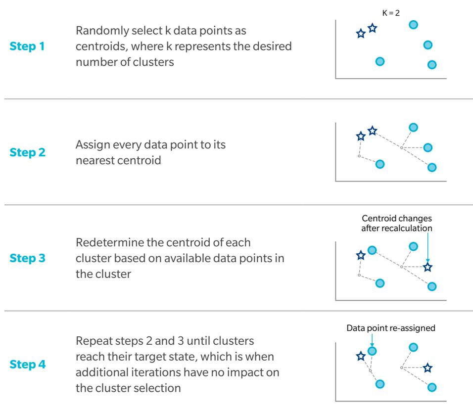
A K-means clustering algorithm is simple to define and illustrate. It partitions the data into a well-distributed set of clusters when k is relatively small. However, this technique can be sensitive to outliers and initial assignment of the k data points.
